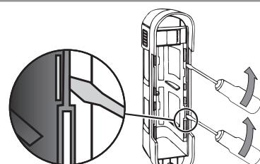
**2** Slide the lens forwards to angle the beam 3° (away from the wall).
