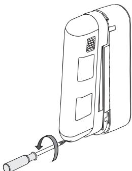
**2** Remove the 2 fixing screws (b) from the base. **Do not touch the mirrors.**
